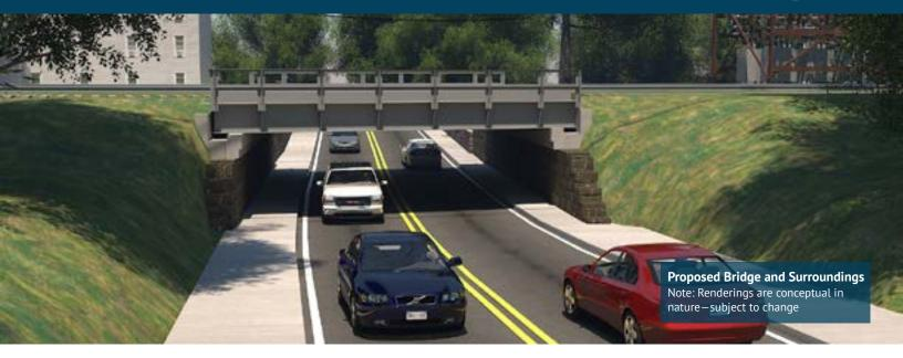
Built in 1894, the Osborne Avenue Railroad Bridge supports four tracks of the New Haven Line. The Program replaces the existing bridge and rehabilitates the supporting structure underneath, while maintaining the current vertical and horizontal clearances. The replacement is built in halves during construction of the Walk Bridge, allowing work to be done during planned two-track outages for the Walk Bridge replacement.
