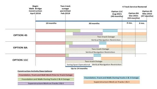
Figure ES-11—Construction Schedule - Comparison of Bridge Options
