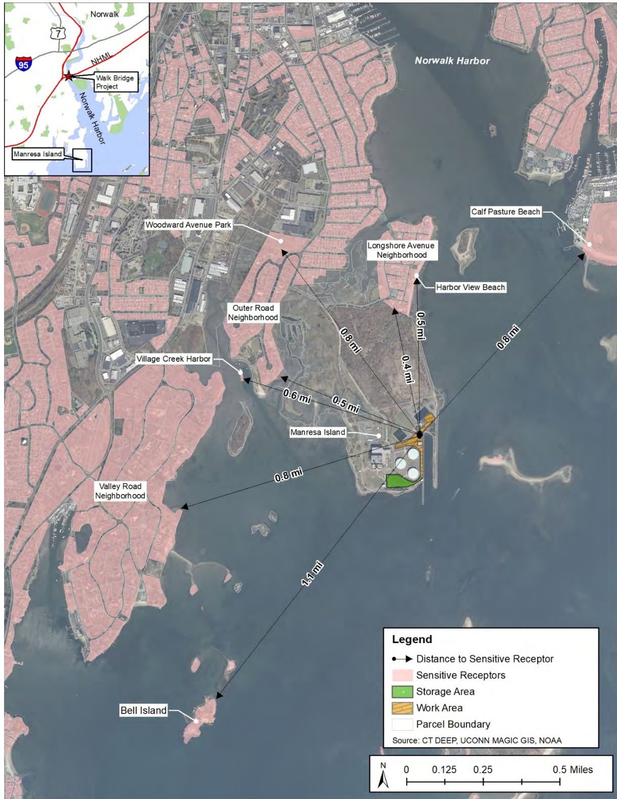
Figure F-2—Proximity of Sensitive Receptors to Manresa Island Staging and Storage Yard
