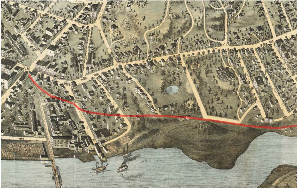
Figure 3: The south end of the Danbury and Norwalk Railroad (shaded) as shown on the 1875 Bailey bird's-eye view. The line runs at street level, with a long siding extending south to the lumber yard and dock at the end of Marshall Street.
